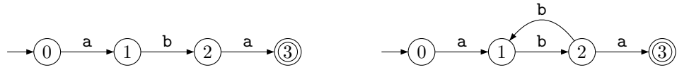
Figure 5. We have the automaton \mathcal{A}_X^0 (left) for X = (aba, abbba) and the incorrect construction of \mathcal{A}_X^1 (right): adding the edge (2, b, 1) would lead to an automaton accepting the infinite language \{aba, a(bb)^*a\} .
